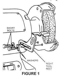
b. Install adjustable rests (22 and 35) to the wheel guards (7 and 27) as
